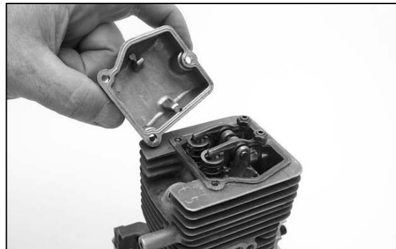
Remove rocker arm cover to expose rocker arms and upper ends of pushrods.
