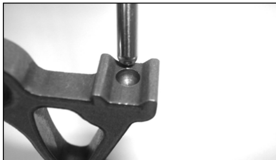
Make sure pushrods are seated in retainer cups in followers and rocker arms upon reassembly.
