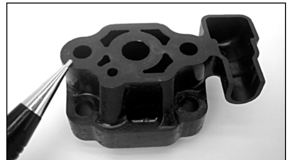
Integrity of carburetor mounting surface is critical to engine performance.
