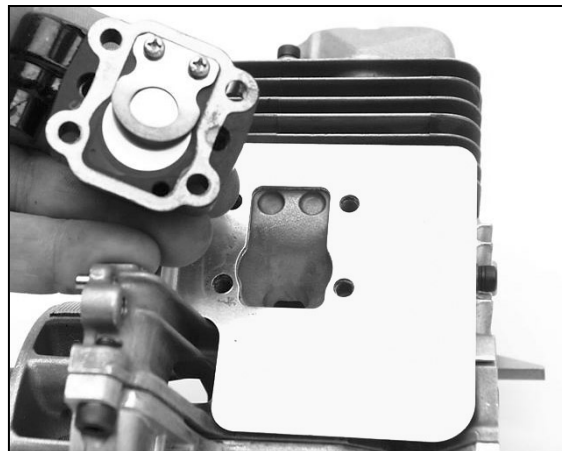
Intake reed valve is mounted on back (engine) side of carburetor insulator block. Reed valve/insulator block must be replaced as a complete assembly.
