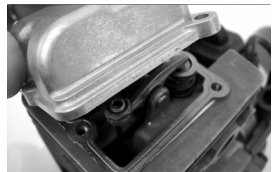
To ensure proper sealing, always use a new gasket when replacing covers.
