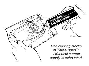
Figure 8.24 Applying Liquid Gasket (not used on Models 488, 575 and 695)
