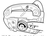
Figure 13.6 Remove the Clutch Assembly
